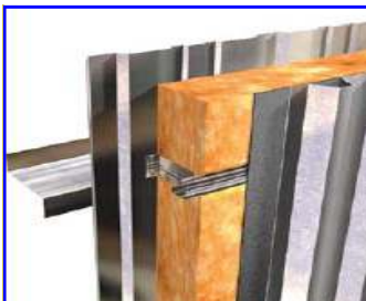
Vertical:- Site assembled Fire Walls
