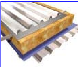
Roof:- Site assembled
