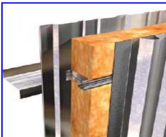
Vertical:- Site assembled Fire Walls
